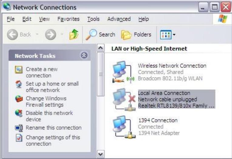
Now you can either right click on the Local Area Connection and select “Properties” or highlight it and click on “Change settings of this connection” from the Network Tasks sidebar, as shown above. When you do this, the following window will open.
