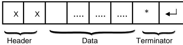
Each command frame starts with a two-byte ASCII character header, followed by a number of ASCII data and ends with a terminator which is comprised of a '\*' character and a carriage return (ASCII value = 13<sub>10</sub>). The header denotes the purpose of the command. For example, RI for Read Input, WO for Write Output, etc. The data is usually the hexadecimal representation of numeric data. Each byte of binary data is represented by two ASCII characters (00 to FF).
