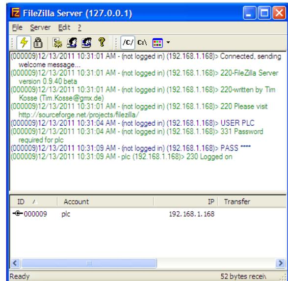
2. Once you get the “230 Logged On” message you know that the FTP setup is done correctly. Note that the welcome message from the FTP Server shows only one line “220 FileZilla Server Version x.xx” which is what we have set it up to be. You can now disconnect from the FTP server by typing “Quit” at the command prompt.
