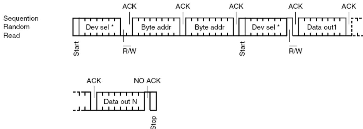
Reading data from a random EEPROM location is slightly more involved than writing. You need to first use the I2C\_WRITE command to set the memory pointer inside the M24M01 to point to the memory address location, then immediately followed by I2C\_READ command to read one or more data bytes
