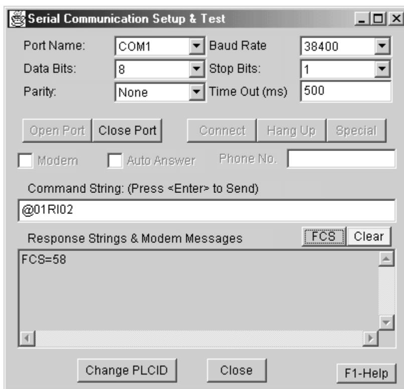
You now can enter the complete command string as "@01RI0258\*" and it will be accepted by TLServer. (Note: If the PLC has executed a `SETPROTOCOL n, 5` to configure its serial port into pure native mode, then wildcard FCS will not be accepted and you must use the actual FCS with your command. The FCS button makes it much easier than computation by hand).
