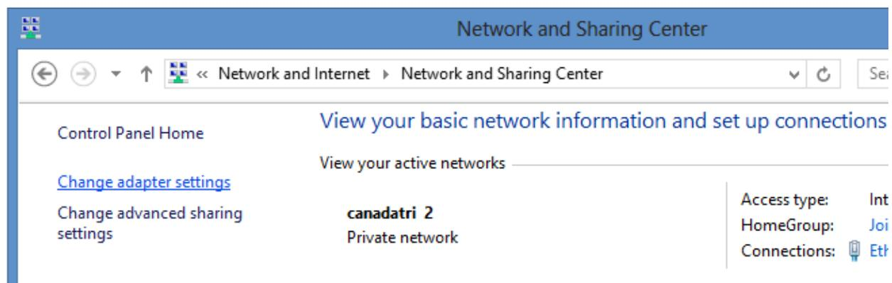
3. **Click on the "Change Adapter Settings" Link.** This will bring up the "Network Connections" window where you can configure the necessary network settings for the local adapter.
