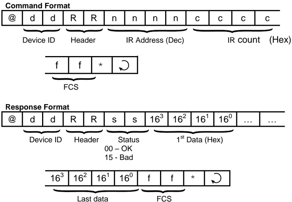
E.g. To read Timer PV #1 to #7 using this command, send:
