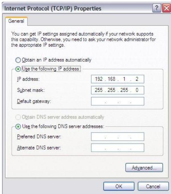
Here is an example of a configuration that will work if your PLC has an IP address of 192.168.1.xxx, where xxx is anything from 1-255 except 2.
