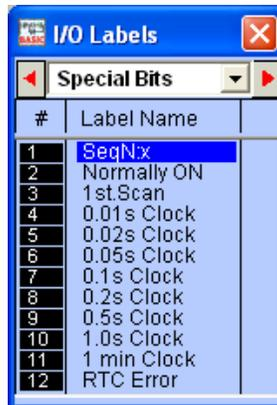
The "Special Bits" table is located after the "Counters" table and before the "Inputs" table. Click on the "SeqN:x" item to insert a sequencer bit. You will be prompted to select a sequencer from a pop-up menu. Choose the desired sequencer (1 to 8) and another dialog box will open up for you to enter the specific step number for this sequencer.
