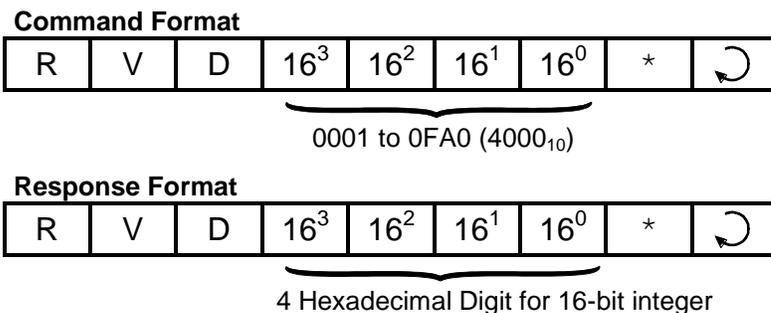
E.g. To read the value of DM[3600], send host-link command "RVD0E10\*". If variable DM[3600] contains the value 12345<sub>10</sub> (=3039<sub>16</sub>), PLC will send the response string as "RVD3039\*".
