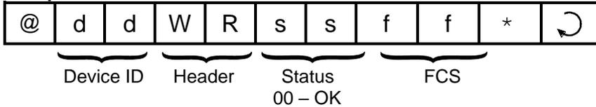
E.g. To Write to CtrPV #1 to #2 using this command, send:
