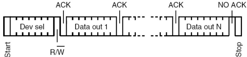
An **I2C\_READ** command begins with the master (PLC) sending the START bit, followed by a 7-bit slave address, and then a "R/W" bit set to high, which indicates that it is a READ command. If the slave device with the targeted slave address is present, it will send the ACK response to the master. Otherwise the master sends a STOP bit and quit the I2C\_WRITE function.
