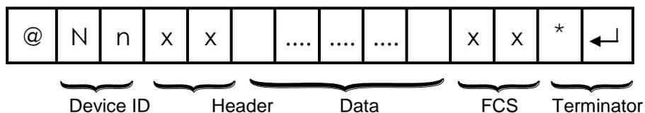
Each command frame starts with the character "@" and two-byte hexadecimal representation of the controller's ID (00 to FF), and ends with a two-byte "Frame Check Sequence" (FCS) and the terminator. FCS is provided for detecting communication errors in the serial bit-stream. If desired, the command frame may omit calculating the FCS simply by putting the characters "00" in place of the FCS.
