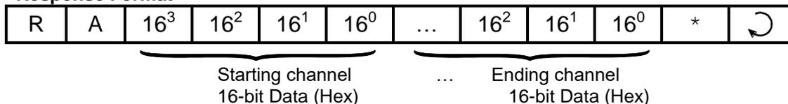
E.g. To read 4 channels of Analog inputs starting from Ch #2, Send "RA0204\*". The response string will contain 4 sets of data for channel 2, 3, 4 and 5.
