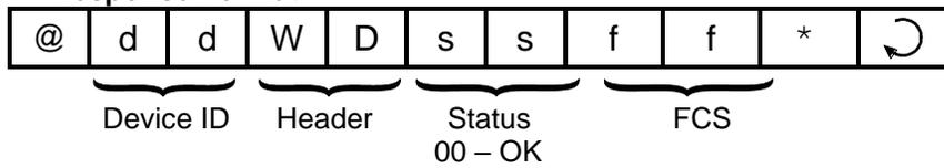
E.g. To Write to DM#1200 to #1201 using this command, send:
