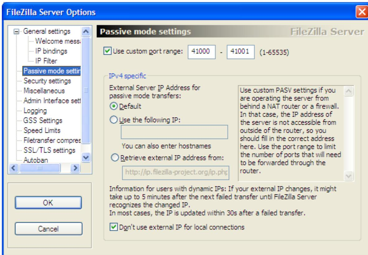
Next, open up Windows Firewall and add to the Exception list the port 21 (command port) and ports 41000 to 41001 (or whatever range limit you have set to in the FileZilla Setup screen). This should allow the FTP Server to receive connection from these ports that the PLC will be using to make the command and data connections.
