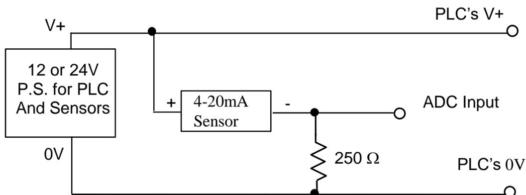
\* For ADC #7 & #8, use a 253.16 ohm resistor instead of 250 ohms as explained in 5.2.2.
