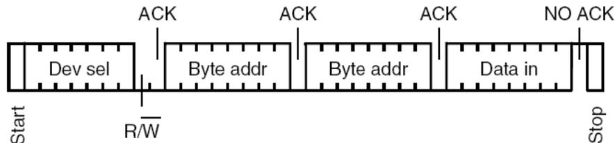
An **I2C\_WRITE** command begins with the master (PLC) sending the START bit, followed by a 7-bit slave address, and then a “R/W” bit set to low, which indicates that it is a WRITE command. If the slave device with the targeted slave address is present, it will send the ACK response to the master on the 9<sup>th</sup> clock cycle. Otherwise the master sends a STOP bit and quits the I2C\_WRITE function.
