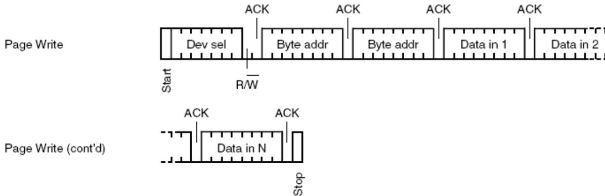
Example. To write 4 byte of data XX to the EEPROM address 19876 to 19879 (&H4DA4) in first 64K bank, you need to do the following:
