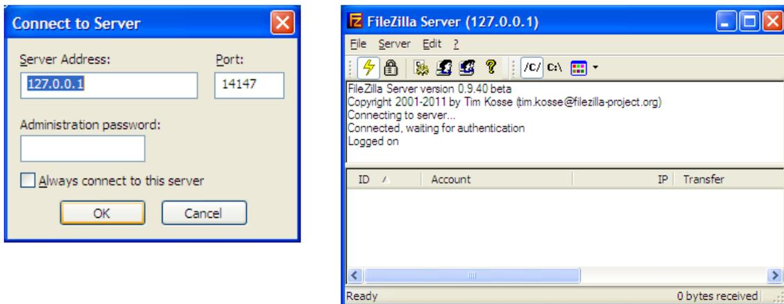
3. If the FileZilla Server is running on the same PC that you are running the FileZilla Server Interface program then you can use the localhost IP address which is 127.0.0.1 – the Port can be anything since this is a client port that the Interface program is using to interact with the FTP Server (don't be confused with the FTP **Server** listening port which is by default = 21).
