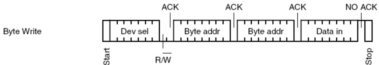
Example. To write a byte of data XX to the EEPROM address 54321 (&HD431) in first 64K bank, you need to do the following:
