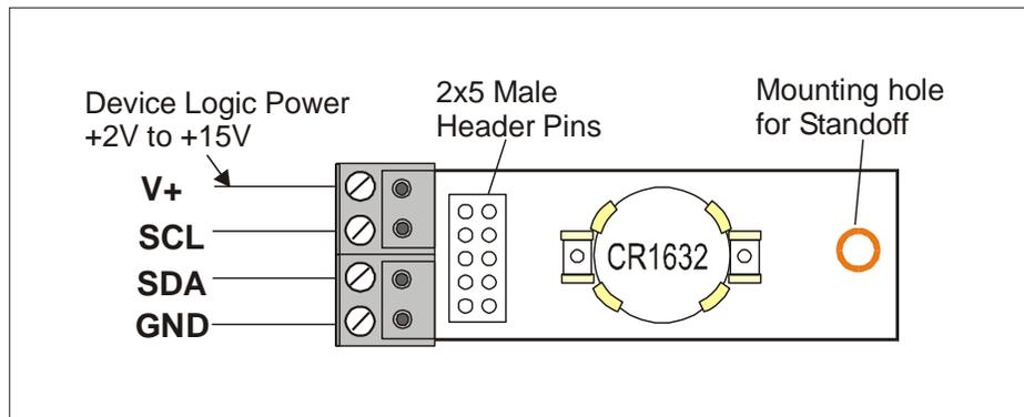
The I2C-FRTC modules adds the following hardware to the FMD1616-10
