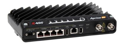
Smart, secure, industry-leading speed licensed point-to-multipoint SCADA communications for industrial monitoring and control for the electricity, water, oil and gas industries - now with 256 QAM
