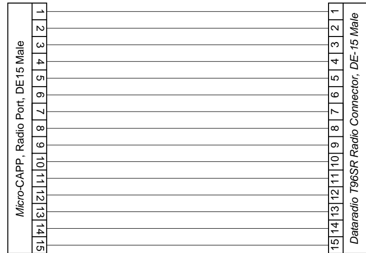
Micro-CAPP to Dataradio T96SR Interface (CABLE B)
